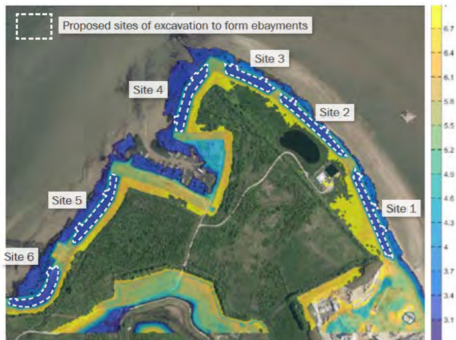
Lidar plan showing proposed ebayment sites to be excavated. These six sites will be reduced in level from 5.5m by circa 2.5m to approximately existing mean high water level and the inter-tidal zone. The proposals will create approximately 2ha of new salt marsh habitat.
