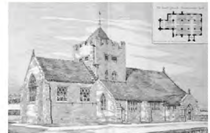
All Saints Church is a local landmark on the junction of Galley Hill and London Road. It designed by Richard Norman Shaw in 1894. Built from knapped flint, typical of the area, it was intended for the workers of the cement industry. It is now residential accommodation. (source: [redacted])
