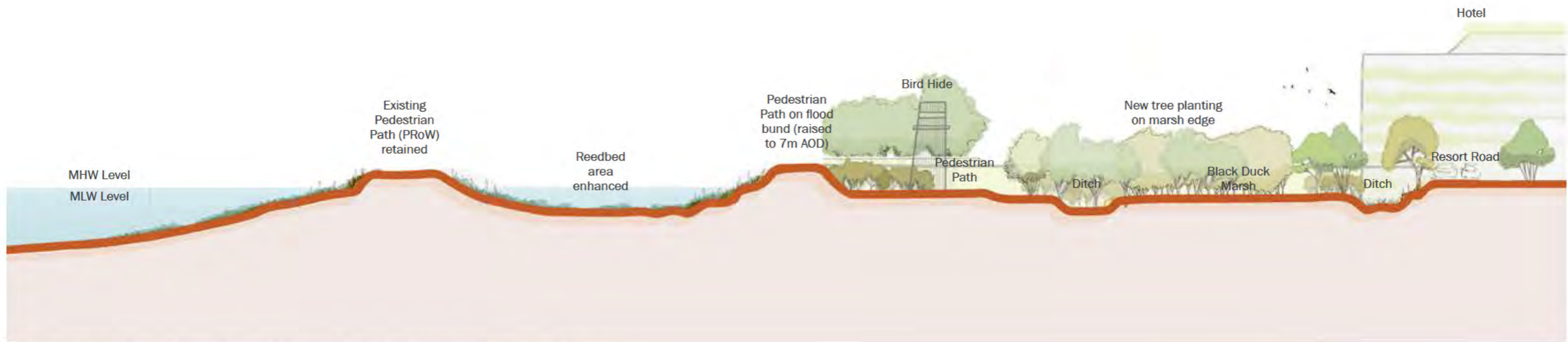
Figure 25. Cross Section through flood defences, Black Duck Marsh Edge and Resort Road
