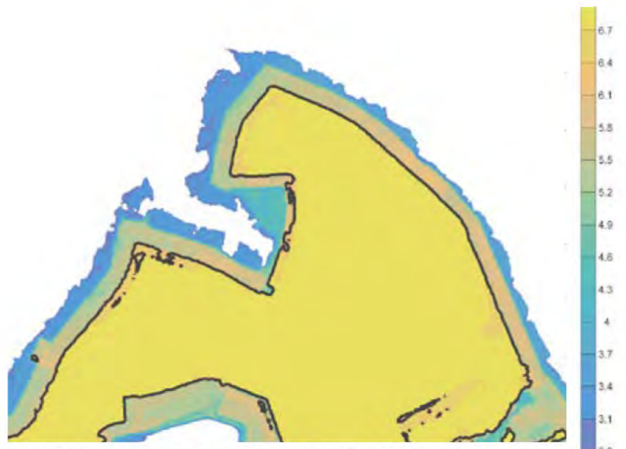
Existing lidar plan, showing existing salt marsh (inter-tidal zone level @ approx 3.5m) in dark blue, river bank terrace in green and higher ground open scrub mosaic in yellow. (NOTE: Detailed ground-truthing of levels is to be completed)
